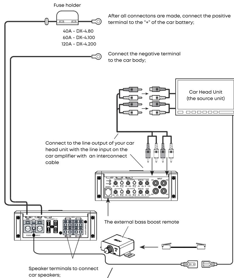
Car amplifier turn-on control wire. Connect this terminal to the corresponding wire on the head unit. The terminal can also be connected to a car antenna resistor. Another way is to connect the turn-on control wire to the car ignition.
