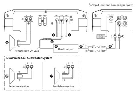
\* If the connected head unit does not have a Speaker Output and RCA Extension Cable (10) cannot be used, you can use the Speaker-RCA Conversion Cable (10) (sold separately). For details on how to make a connection, see "About Connecting to the Speaker Input Level System" (page 14).
