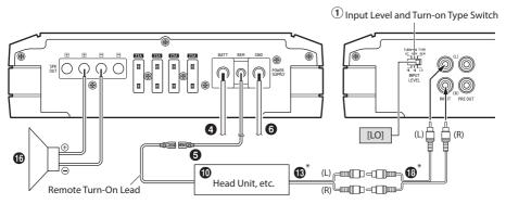
\* If the connected head unit does not have a Speaker Output and RCA Extension Cable (18) cannot be used, you can use the Speaker-RCA Conversion Cable (19) (sold separately). For details on how to make a connection, see "About Connecting to the Speaker Input Level System" (page 14).
