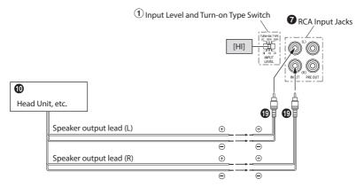
• Do not mistake the Speaker Output Lead on the head unit side connected to this unit.
