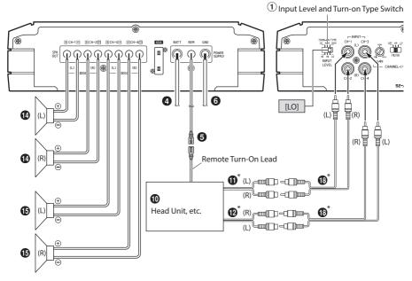
\* If the connected head unit does not have a Speaker Output and RCA Extension Cable (10) cannot be used, you can use the Speaker-RCA Conversion Cable (10) (sold separately). For details on how to make a connection, see "About Connecting to the Speaker Input Level System" (page 16).
