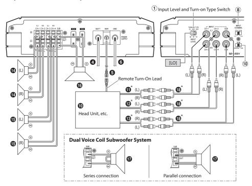
\* If the connected head unit does not have a Speaker Output and RCA Extension Cable (19) cannot be used, you can use the Speaker-RCA Conversion Cable (19) (sold separately). For details on how to make a connection, see "About Connecting to the Speaker Input Level System" (page 16).
