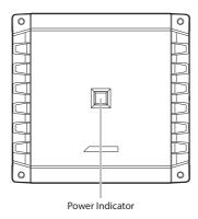
Lights up when power is on. Is off when power is off.
