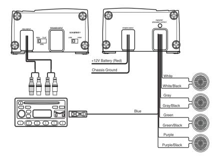
In this application, the XC1410 is used as a 4-channel amplifier to drive four full range speakers in stereo. This configuration is for headunits with RCA outputs.
