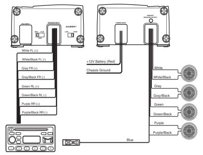
In this application, the XC1410 is used as a 4-channel amplifier to drive four full range speakers in stereo. This configuration is for headunits with High Level Speaker Outputs. Please note: this configuration is also for Factory OEM headunits.
