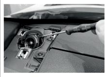
Then remove the original connection of the tweeter. Press the release button to unplug the connector.
