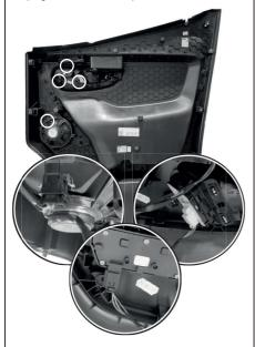
When every clip, lever and electrial connection is unhooked, unhook the door panel from the two lower hooks on the door. Tilt the door panel away from the door and lift upwards.
