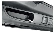
Use a small flat head screwdriver to remove the plastic cover. Be careful and avoid to make ant notches. Unscrew the torx.
