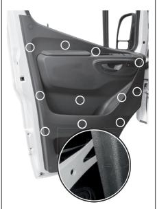
When all clips are released, you need to press out the door pin in the upper area of the trim. Push the pin and the plate in the direction of the window (away from you).
