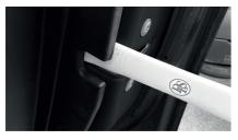
When the door panel is loose, start by softly lifting the panel straight up to remove it.
