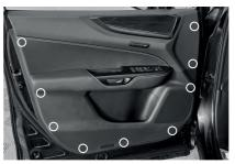
Usually the clips/screws are placed by the white marks. This could vary depending on the vehicle.
