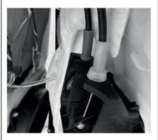
Disconnect electrical connections for the door lights.
