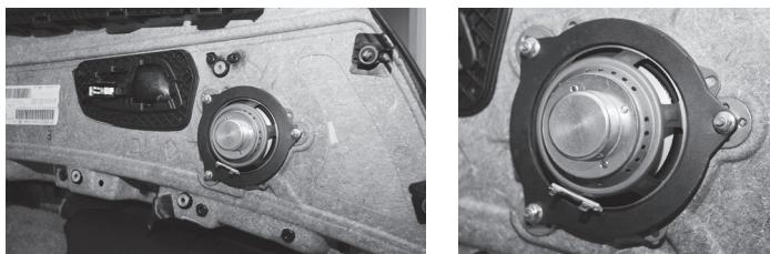
The tweeter (RC25) fits directly in the A-pillar tweeter attachment but we recommend the use of hot melt glue to secure it to the surface.
