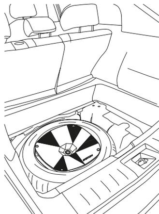
Secure the subwoofer to your vehicle's existing spare wheel mount using the supplied mounting screw & retaining rings, if applicable. Make sure the subwoofer is properly bolted and secured. The wired remote control can be used to adjust the subwoofer, or use the supplied shorting plug to disable the remote control and control your subwoofer using your headunit.
