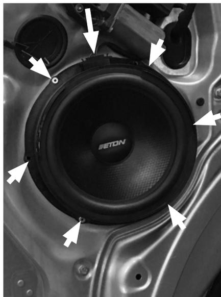
After installing the bass-midrange speaker, fit the rubber sound conduction, available separately by VW, for optimal coupling to the door panel.
