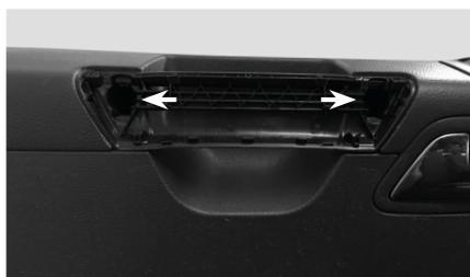
Loosen the Torx screws behind it. There is another one next to the speaker grille (see arrow) and in the below part of the doorpanel.
