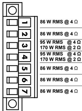
**ATTENTION:** The STEALTH 7.1 DSP has an asymmetrical power distribution. This allows an optimal distribution of the amplifier power to the individual channels. Therefore, when connecting the loudspeakers, make sure that you use the asymmetrical distribution in a sensible way. Channel 3/4 are high-power connections and have more power, so it is advisable to connect bass and midrange drivers to these channels!
