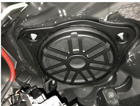
The mounting is carried out with the 3 factory fitted M6 nuts. Take care not to tighten the nuts too tightly, for M6 a tightening torque of 8-10Nm applies.
