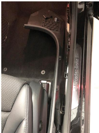
The front basses are fixed with 3 M6 nuts (nut size 10). The fairing parts or component carriers placed above them are also fastened with M6 nuts or Torx sheet metal/plastic screws.
