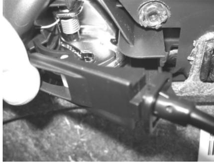
Loosen the plugs for window regulator and other features. Pry possibly remaining clips out of the door and re-insert them in the door paneling.
