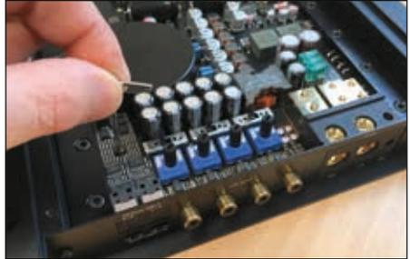
7. Fix the new side panel which is delivered with the HDM 1 module with the Allen screws. Afterwards remount the acrylic cover, too.
