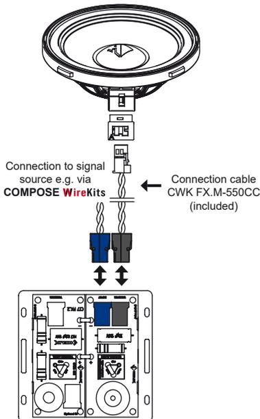
**Option d:** Direct connection to OEM connector with optionally available **FlexConnect** inlay
