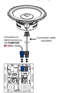
Ensure that all components are correctly connected in polarity, i.e. plus to plus and minus to minus. The positive leads of the loudspeaker system are marked red.
