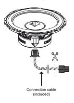
Option b: Universal connection to the blade terminals via optional car-specific harness or COMPOSE
