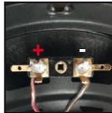
**Ensure that all components are correctly connected (phase), i.e. plus to plus and minus to minus. The positive leads of the loudspeaker system are marked with a red stripe.**
