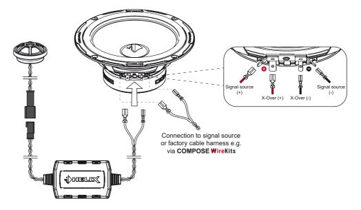
Ensure that all components are correctly connected (phase), i.e. plus to plus and minus to minus.
