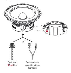
Ensure that all components are correctly connected in polarity, i.e. plus to plus and minus to minus. The positive leads of the loudspeaker system are marked red.
