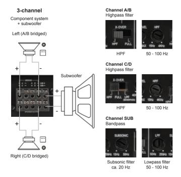
Note: The values listed here are empirical values that have been approved as useful in practice. Depending on the size of the loudspeaker we recommend the following highpass filter settings: ca. 50 Hz for 6.5"/16.5 cm LS; ca. 70 Hz for 5.25"/13 cm LS; ca. 100 Hz for 4"/10 cm LS
