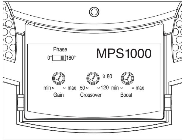
**Power LED:** This indicator will glow blue when the MPS1000 is operational.
