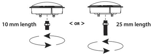
Stud bolts are provided in two lengths to accommodate different panel thicknesses.
