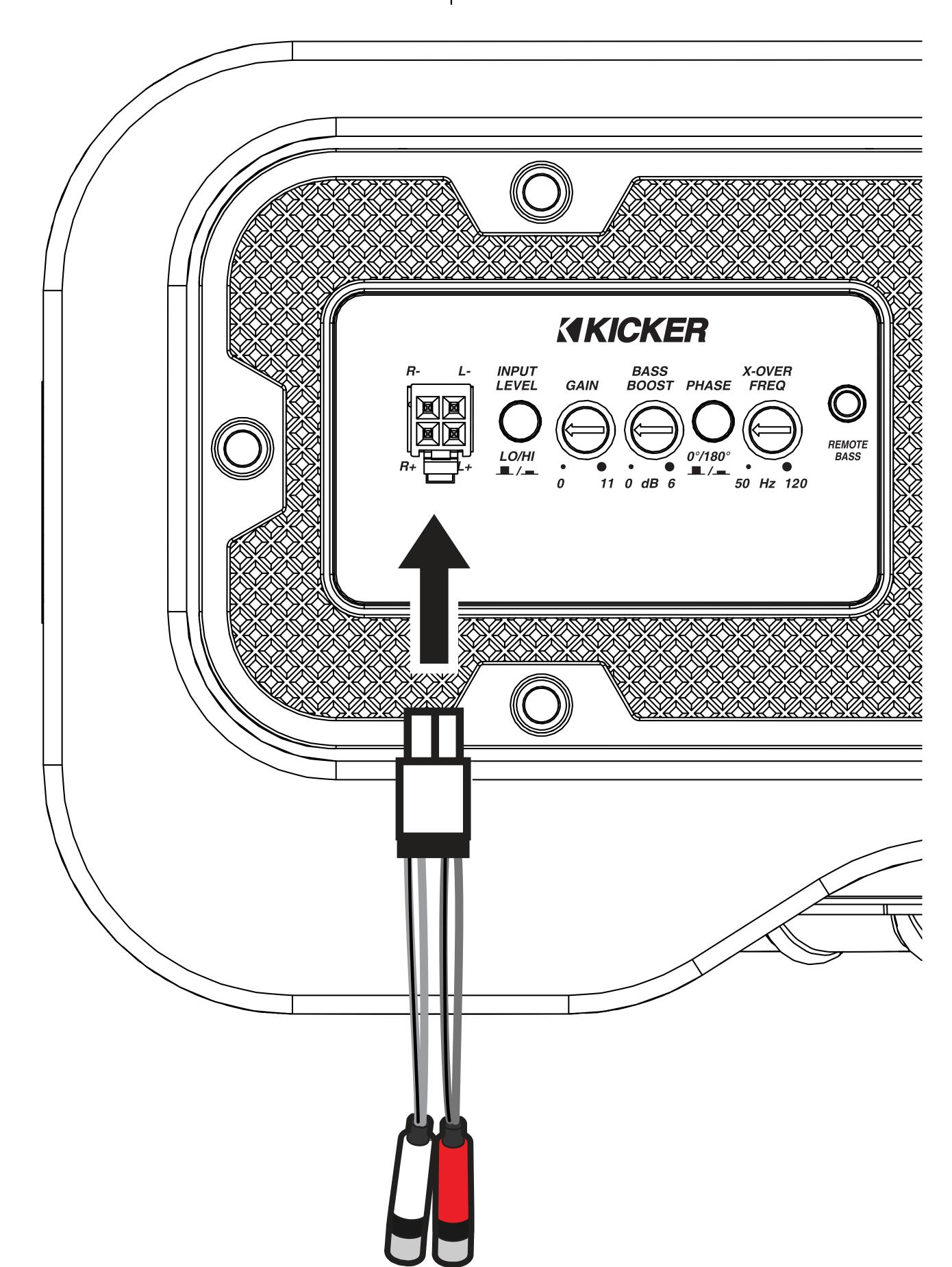
If needed, cut off the RCA connections to use hilevel input, or use the <u>KICKER KISL Speaker-RCA</u> Converter.
