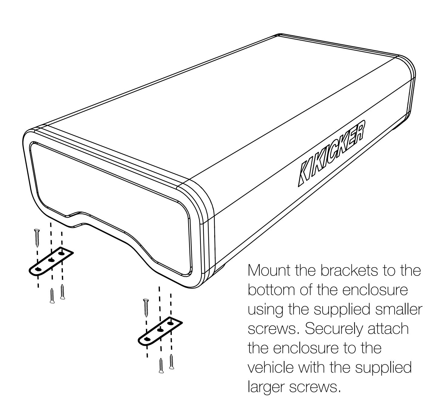
If the supplied mounting hardware is not applicable to your installation, some other means of securely attaching the enclosure to the vehicle must be used.
