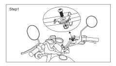
1. Install "P" shaped clamp (item#2) or "Z" shaped bracket (item#3) threaded on to the Bluetooth controller hook. ( packed with Bluetooth controller). Use the provided bolt (item#10) to fix on the handlebar, it can be adjusted the tightness by provided EVA & rubber pad.(item#7)
