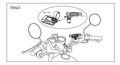
2. Slide the Bluetooth controller into the hook.
