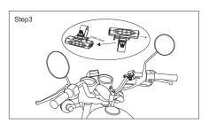
3. Press down the Bluetooth controller hook and then slide out the Bluetooth controller box at the same time to remove the the Bluetooth controller.
