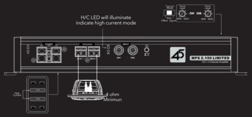
Fuses must be positioned to inner fuse holders labeled "High Current" to maximize output power when connecting a 4-ohm mono speaker load
