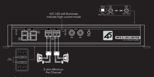
Fuses must be positioned to inner fuse holders to maximize output power when connecting a 2-ohm speaker load
