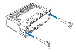
3 Install the sleeve into the dashboard and bend the tabs outward to fix the sleeve.
