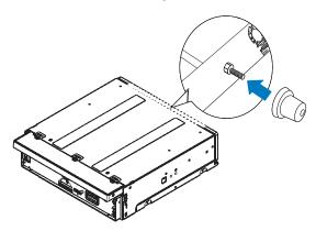
Install the sleeve into the dashboard and bend the tabs outwards to fix the sleeve. Slide the unit into the dashboard until you hear a click.
