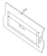
3 Install the sleeve into the dashboard and bend the tabs outward to fix the sleeve.
