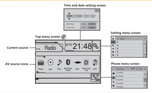
By pressing the ## button on any screen you can display the Top menu screen.
