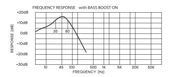
NOTE: Raising the Bass Frequency allows higher frequencies to reach the bass speakers centered around 45Hz. This "BUMP" can have a dramatic effect on the bass system's apparent volume. Use caution! When adjusting this control as serious subwoofer damage may result from overpowering or overexcursion.
