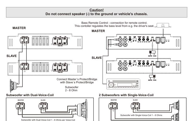
Caution: Please observe the right polarity. Slave's - to Loudspeaker's + and Slave's + to Loudspeaker's -.
