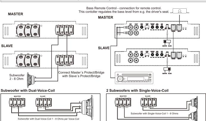
Caution: Please observe the right polarity. Slave's - to Loudspeaker's + and Slave's + to Loudspeaker's -.
