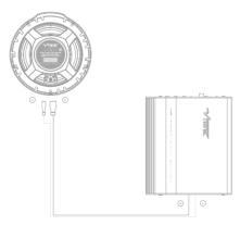
• Connect the speaker to the speaker wiring in the vehicle ensuring that correct polarity is observed.
