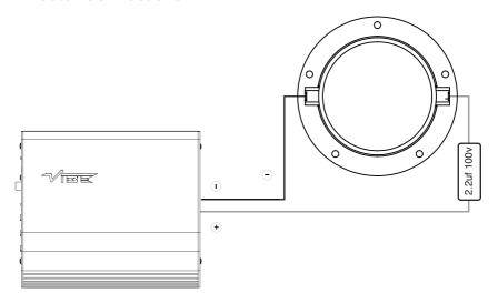
**NOTE:** Unless using an active crossover network, the 2.2uf 100v capacitor must be fitted in order to avoid damage to the tweeter.
